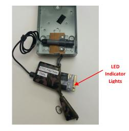
4. When operating normally, the **RED** LED indicator light (see below) should flash once every 5 seconds. The GREEN light should flash when, and only when an object passes the counter. Wave your hand in front of the sensor to make sure it is working. Do not touch the exposed metal contacts:
