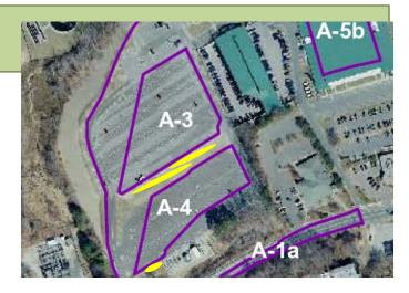
Figure 1. Drainage areas to proposed bioretention cells.
