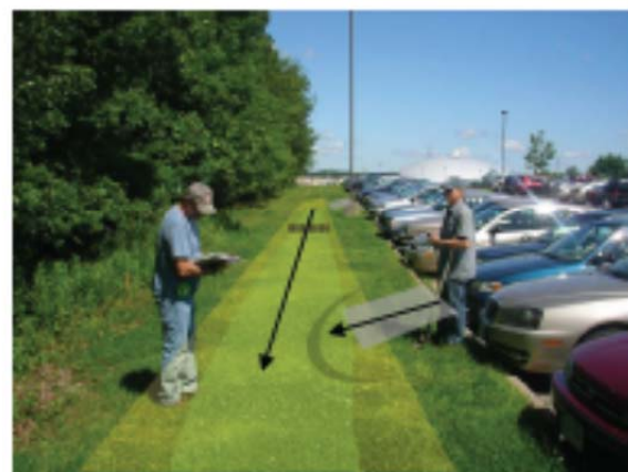
Figure 2. Proposed location of bioretention/swale system in grassed edge of Parking Lot Y. Curb cuts allow inflow to forebays at strategic locations along system.
