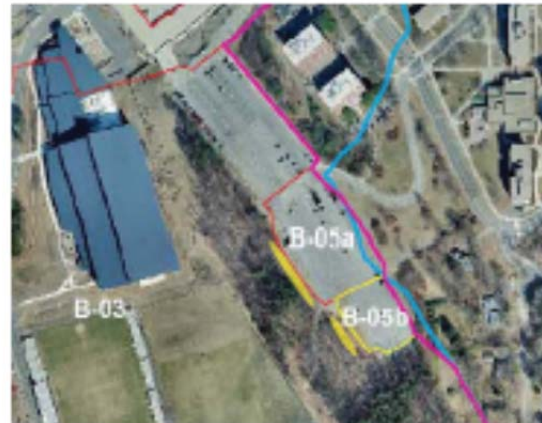
Figure 1. Drainage areas to two proposed bioretention cells.
