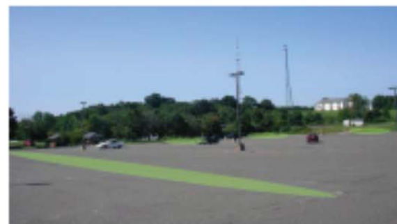
Figure 2. Approximate location of proposed bioretention cells in parking lot. Restriping of lot will be required around landscape island bioretention to alter current traffic flow patterns. Loss of only four or five spaces anticipated.
