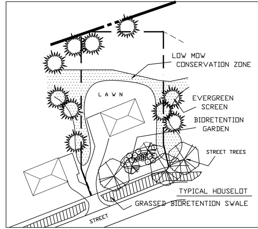
THESE PLANS AND DETAILS WERE PREPARED FOR A SPECIFIC PROJECT. CONCEPTS AND PRINCIPLES MUST BE ANALYZED BY APPROPRIATE PROFESSIONALS FOR ANY OTHER PROJECTS.
